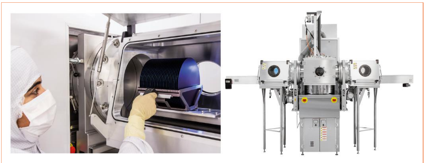
Figure 5: PICOSUN® P-300BV, an example of an ALD reactor developed specifically for LED applications (images credit Picosun)
