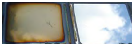
Figure 6: Uncoated (left) vs ALD-coated silver mirror (right) aged four years at room temperature and moisture (image credit Picosun/Dr. Tero Pilvi, doctoral dissertation, University of Helsinki, 2008)
