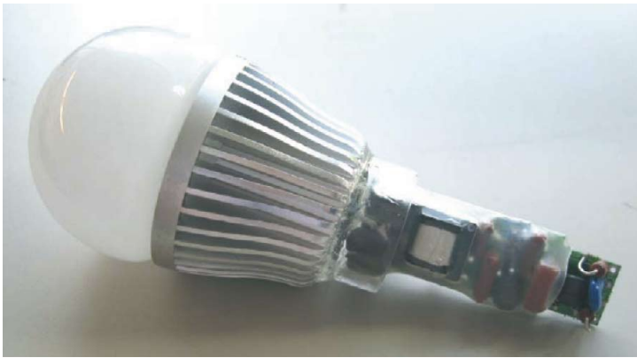
Figure 12: Driver incorporated in an A19 LED replacement lamp (board removed from housing).
